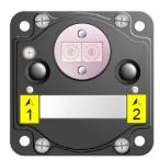
Press the left button (#1) until the display reads \*SITE then, press the right button (#2) to enter the Site Survey menu.
