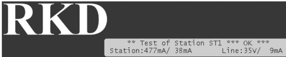
In this case the station pulled a current of 477mA during the "inrush" period, which is when the station is activating the solenoid, and a current of 38mA once the solenoid was open. Numbers in this range are normal; it takes a larger charge in the "inrush" period to pull the solenoid open, and then a smaller current to keep it open afterwards.
