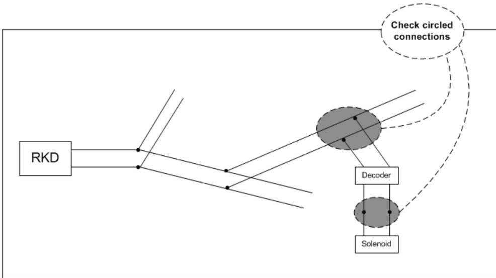
**Figure 8.2. Testing the path to a station**
