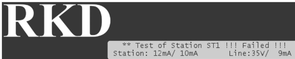
Note how the current during "inrush" and afterwards are practically the same - the station or the solenoid isn't responding.
