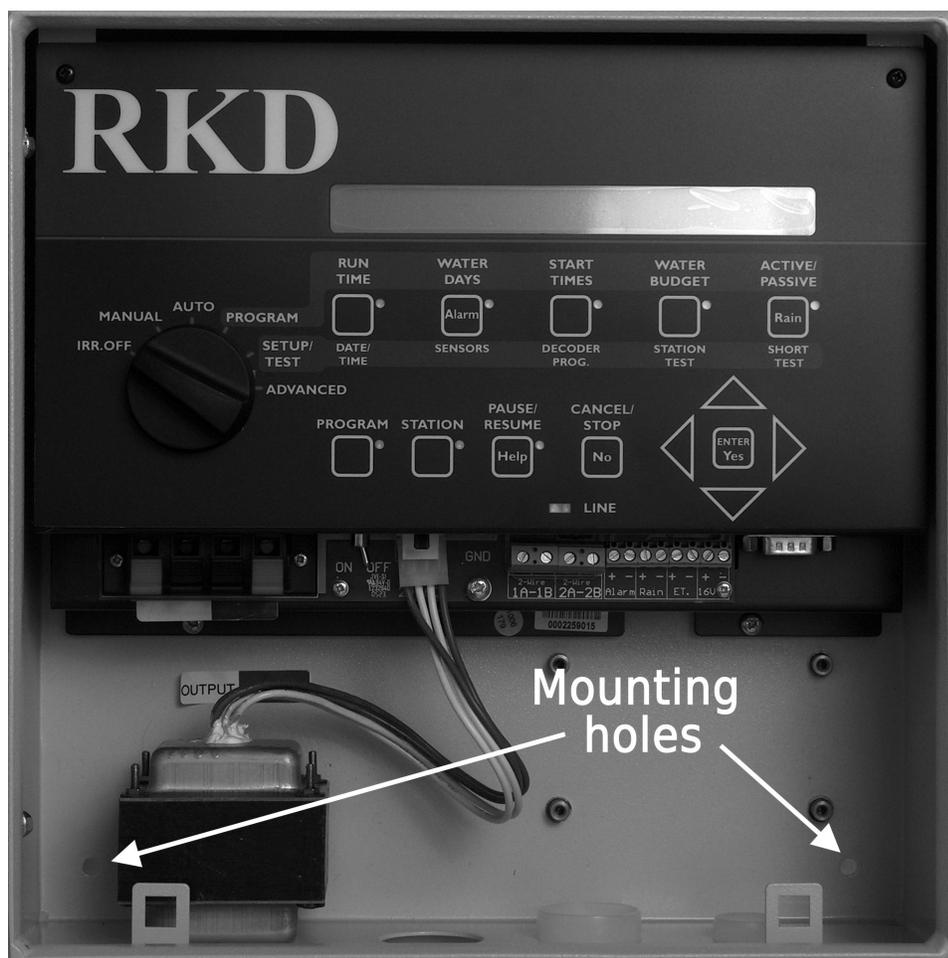
5. If you're placing the controller on a concrete wall, take down the controller, drill out the holes for the two new screws, put in the wall anchors, and put back the controller on the wall.
