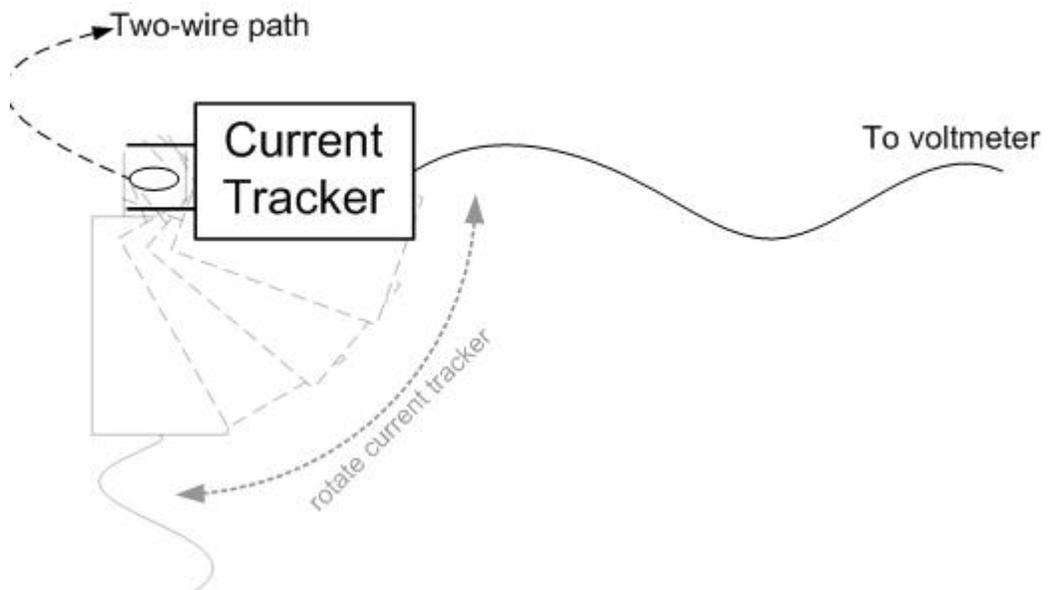
Ideally, you should rotate the current tracker around the individual wires inside the two-wire - do this if enough plastic is stripped off the two-wire.
