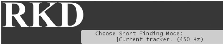
If you just want to view the voltage and current without following up with a field test, it doesn't matter which you choose. But if you want to follow up with the current tracker or a clampmeter in the field, select the setting for the tool you are going to use.
