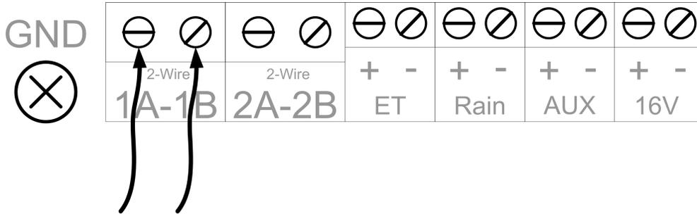
There's room for connecting two cables directly to the controller - the other line can be connected to the terminals labeled 2A-2B. Both wires will receive the same signals when the controller is up and running.
