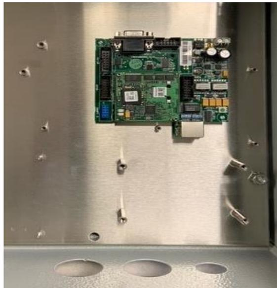
2. Two hex standoffs, two M3 screws, hex spacer nut, and one M4 screw.
