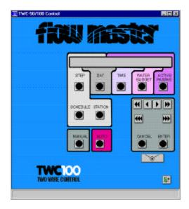
Enter the menus of the controller by clicking the button. The display will show exactly what is shown in the display of the controller on site. The two buttons "Cancel" and "Enter" will be flashing, as they will be activated on the controller on site, to show that the controller is worked on remotely. For information on how to work the menus on the controller, please refer to the controller manual.
