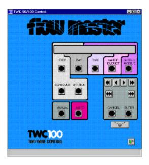
Having connected to the controller, the faceplate of the controller will be shown on the screen. The display will show exactly what is shown in the display of the controller on site. The two buttons "Cancel" and "Enter" will be flashing. Click the "Auto" button with the mouse. The "Auto" and the "Schedule" buttons will be flashing as well. Click "Auto" again to take controller out of auto mode. Click the little green door to disconnect.
