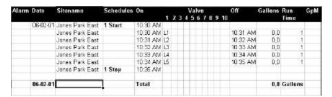
As the example above shows the chosen site is "Jones Park East". Schedule 1 ran Febrauary 6<sup>th</sup> 2001 from 10:30AM to 10:35AM. The schedule consists of 5 steps with one decoder per step. Each step has a run time of 1 minute. In the above case no flow measurements were taken, therefore 0,0 GPM.
