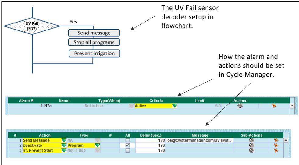
**Figure 33:** The alarm and actions of the UV Fail sensor decoder.
