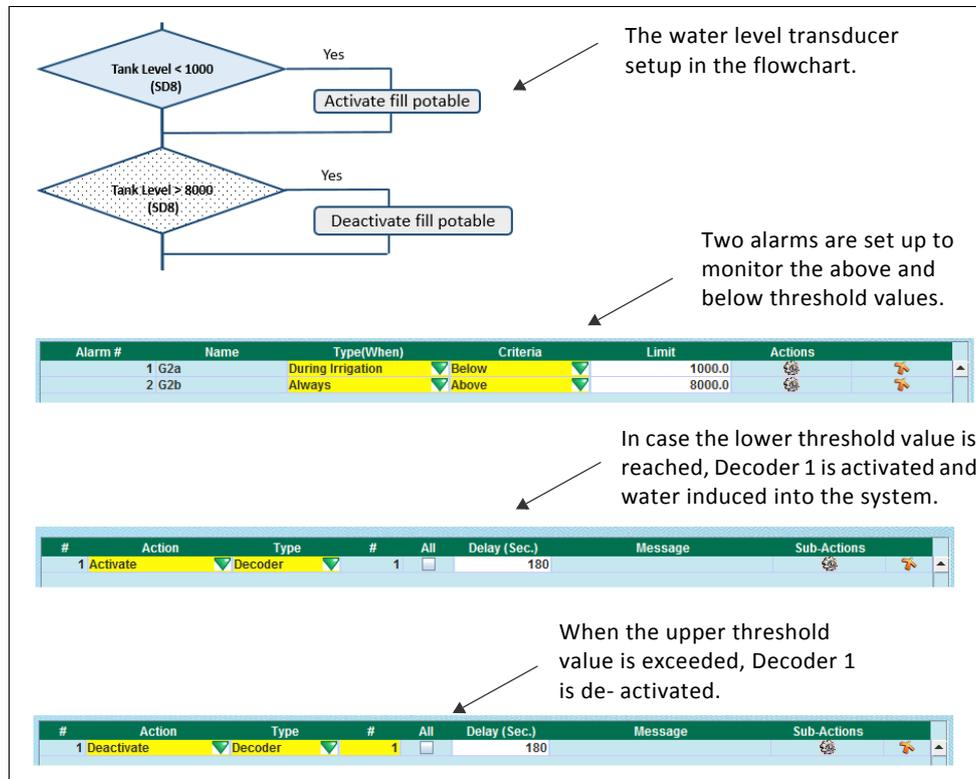
**Figure 36:** The alarm and actions of the water level transducer.
