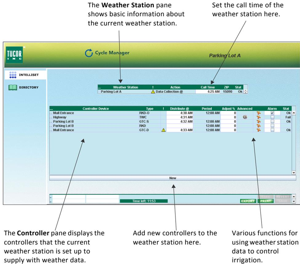
**Figure 39:** The weather station **INTELLESET** window.
