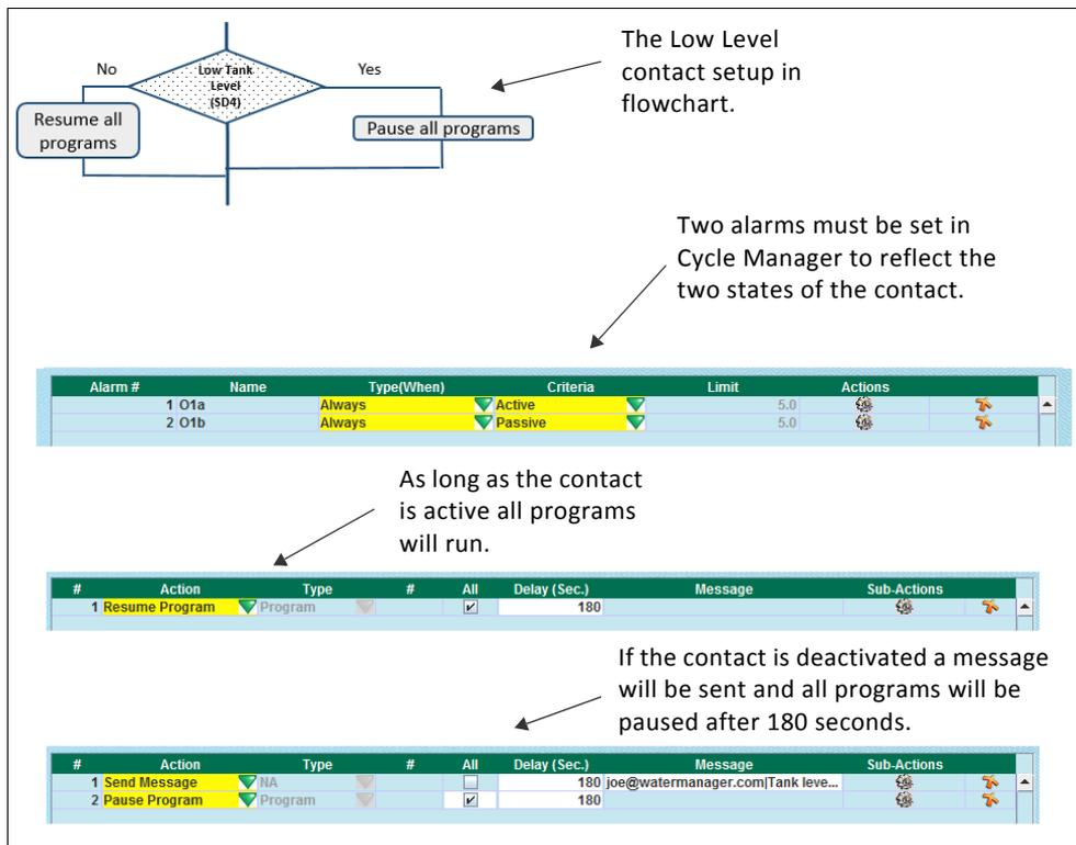
Figure 34: The alarm and actions of the Low Tank Contact.
