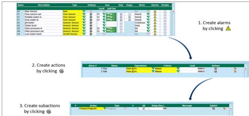
**Figure 28:** The flow of creating alarms, actions and subactions in Cycle Manager.
