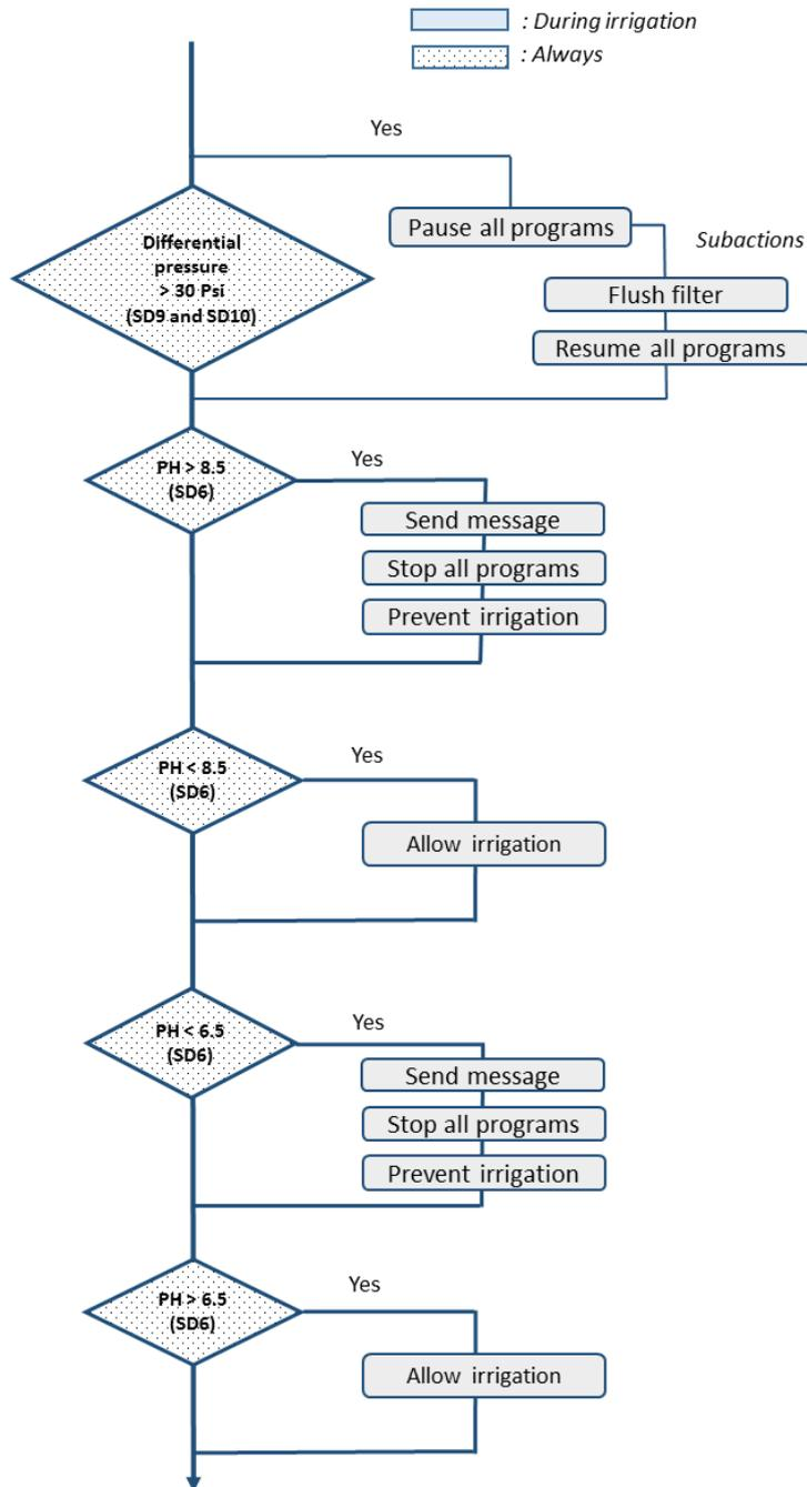
Figure 31: Greywater system flowchart (Part 2).
