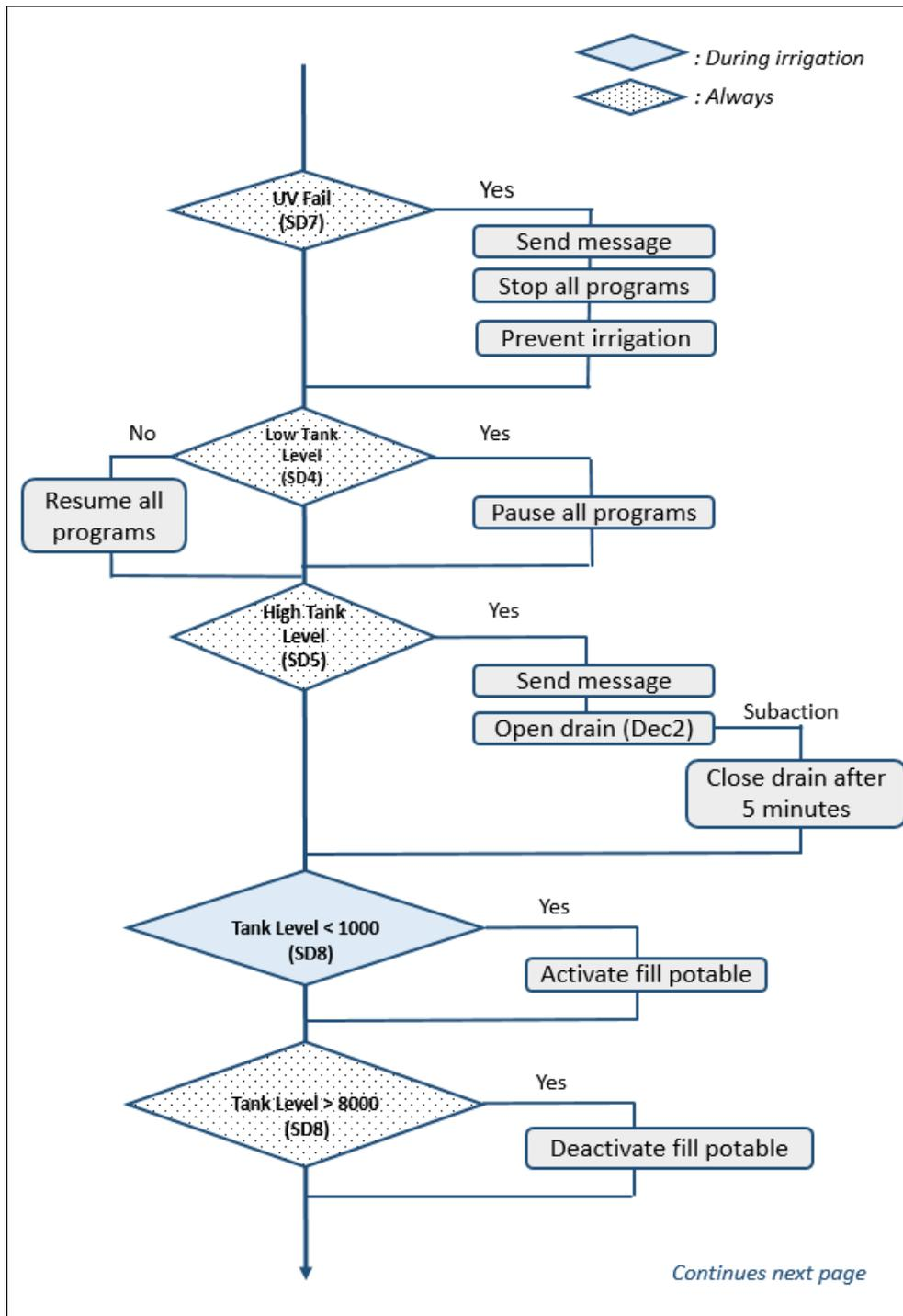
**Figure 30:** Greywater system flowchart (Part 1).
