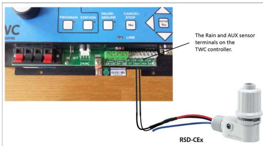
**Figure 20:** A rain sensor connected to the onboard Rain sensor terminal.
