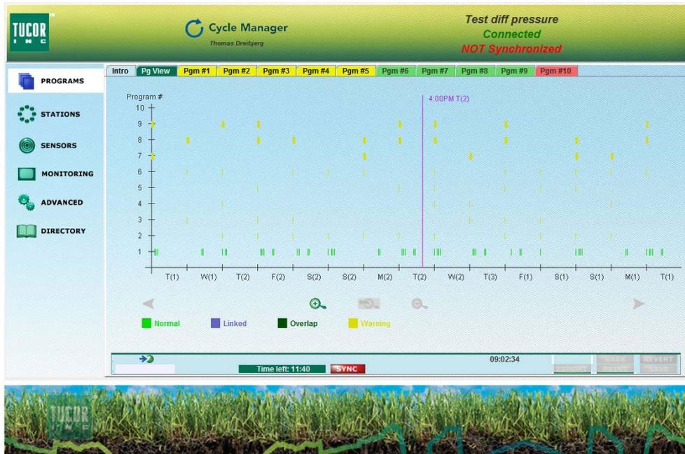
**Figure 16:** The **Pg View** tab provides a simplified graphics representation of all 10 programs.
