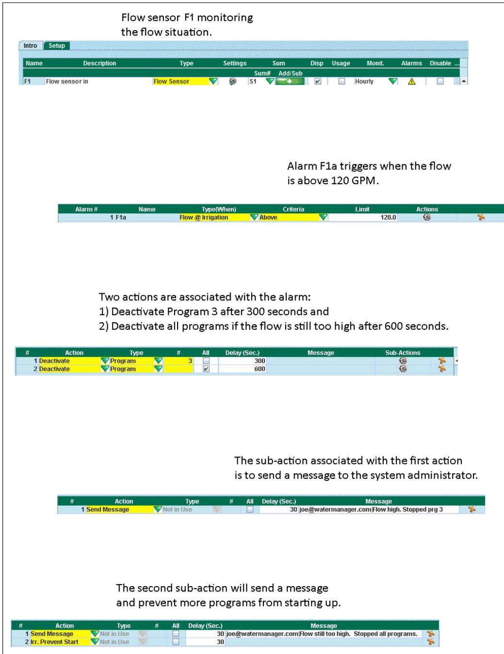
Figure 27: The relationship between and alarms, actions and sub-actions.
