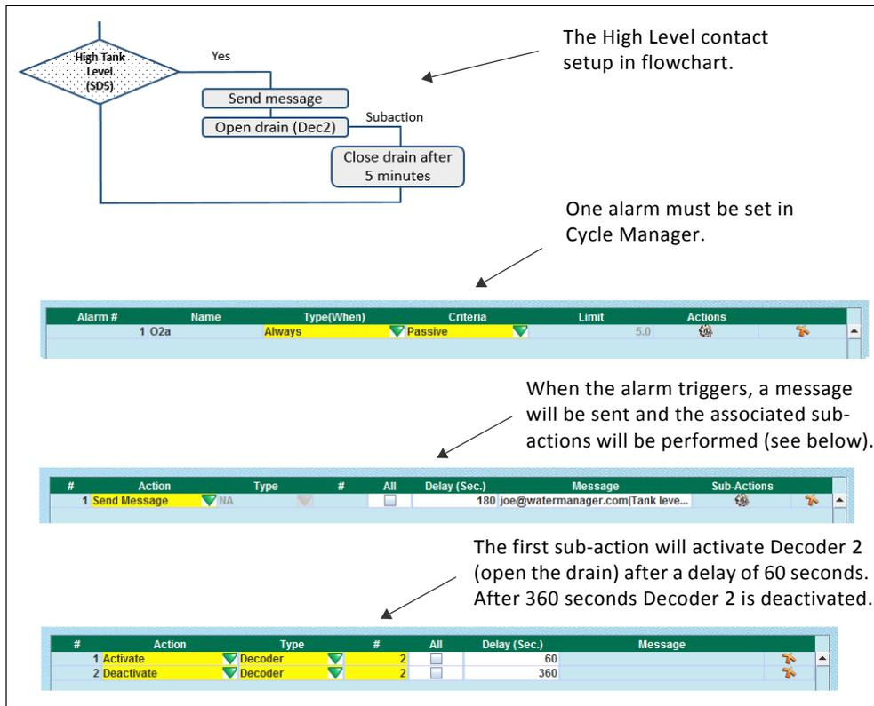
Figure 35: The alarm and actions of the High Tank Contact.
