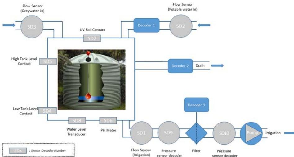
Figure 29: Greywater recycle system.
