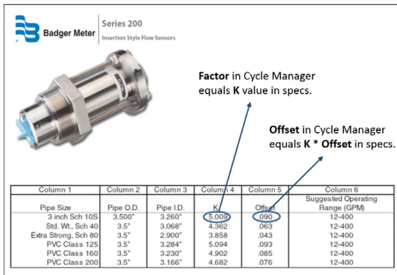
**Figure 26:** Determining the Factor and Offset values from a Badger Meter, Series 200 Insertion Style Flow Sensor.
