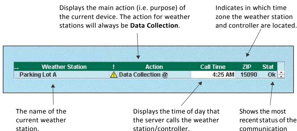
**Figure 40:** Contents of the **Weather Station** pane.
