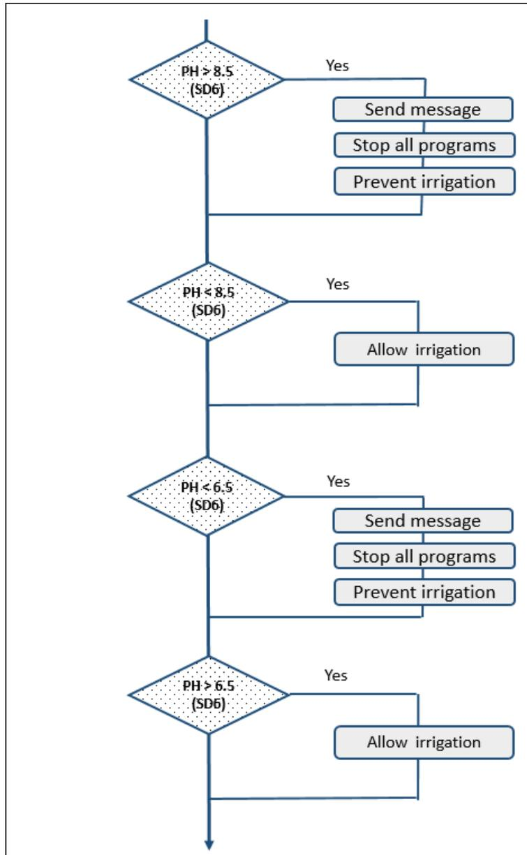
Figure 37: The pH Meter alarms and actions in the flowchart.
