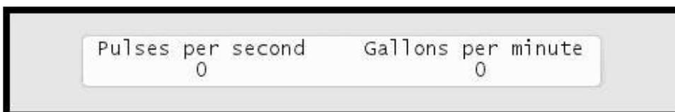
**Note:** The RKS+ can measure correctly up to a flow of 250 pulses per second. If your flow exceeds this you should use a sensor that has a higher "water amount per pulse" ratio. However, a higher frequency is to prefer over a lower one, as it provides the most accurate measuring, so in an ideal world your frequency closes in on 250 pulses per second without ever exceeding it. For more information turn to **Chapter 2: Selecting Sensor Type** on page 31.
