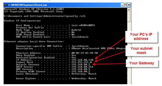
iv. You now need to find an available IP. Obtain, install (but do not update), and run the Netscan program. This will scan your network for available IPs. Enter the IP ranges to scan through as found in the last step and click the "Start Scanning" button. Choose an IP that is not in the displayed list, that is, the last set of numbers must be unique to your LAN. That set will usually be from 000 – 254, so any number within that will work. We recommend using a number in the 040-059 range.
